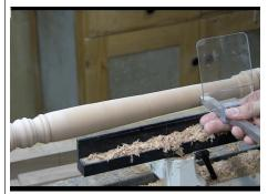
Using your roughing gouge or skew turn the taper connecting the top and bottom then finish off everything with a light sanding.
