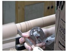
Using a parting tool turn to the desired diameter at each element. Set your calipers from the template itself for this task.
