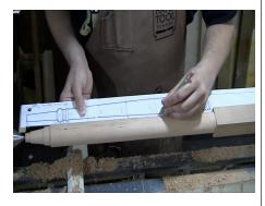
Use the template to mark the location of all the elements on the legs including intermediate points of the taper
