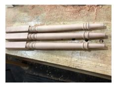
Repeat the layout and turning of each section just as with the first leg and creating duplicates will be much like a paint by numbers. Consistency in process is key.
