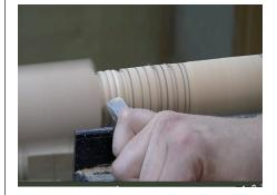
Using a skew chisel roll the beads then coves for the top section above the taper. A skew is necessary to reach between the tightly spaced beads.
