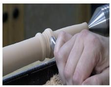
Use the skew chisel to turn the lower beads and foot taper.
