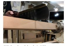
With a leg blank 2-3" longer than needed chucked into the lathe (use a chuck not a drive center) mark the pommel transition and use a saw to sever the fibers on all 4 faces.
