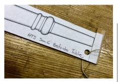
Print out the full sized PDF drawing and mount it to plywood or stiff cardboard using spray adhesive. Include a tab at the bottom of the drawing to act as a fence so you can repeatedly layout the leg on each blank
