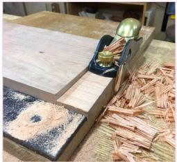
Cut wide tenons on the sides and back of the case and then use a fret saw to cut them into double tenons to allow for wood movement with these wider sides. Chop the mortises to the full width at 1/4" deep then deepen to a full 1" at the double tenon locations.
