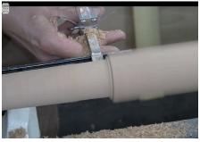
Turn the leg below the pommel to a cylinder equal to the maximum diameter on the template (the top beads)
