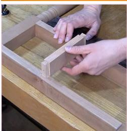
The center and horizontal drawer blades can be milled and dovetails cut so that shoulder perfectly fits between the rails. Start with the vertical divider and fit it into a sliding dovetail first.
