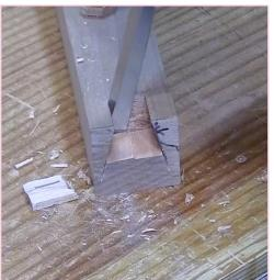
The top front rail is half blind dovetailed into the top of the legs.
